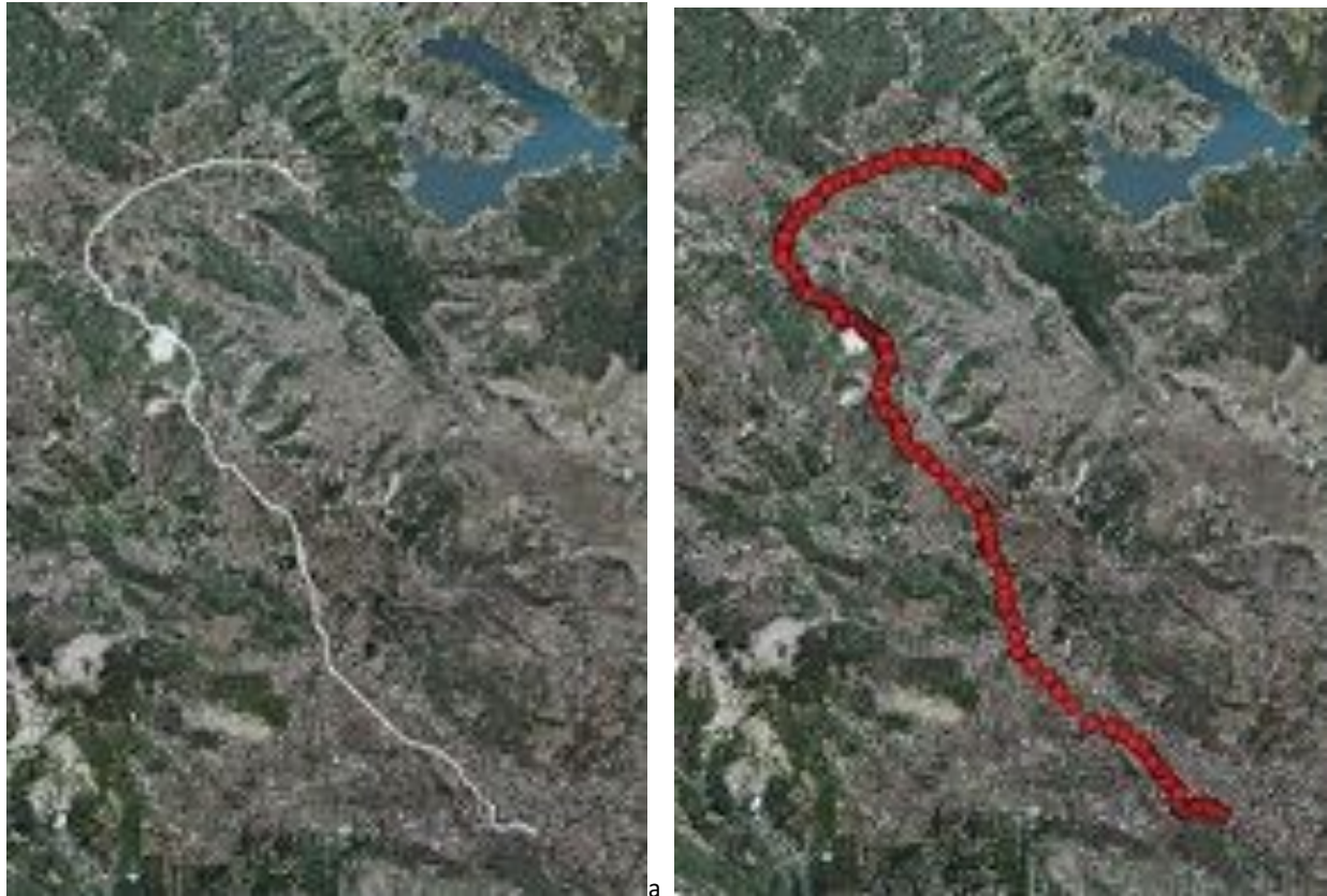
Fig.3. Broken line (a) and corresponding discretization (b) of the rail track on the ortophoto (aerial photography maps)
